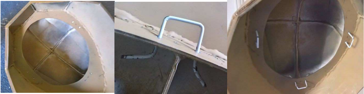
From left to right: 1. The holes drilled for the wire mounting points. 2. One of the pieces of wire inserted into the holes and bent to prevent it from falling out. 3. All three wire mounting points in place.
